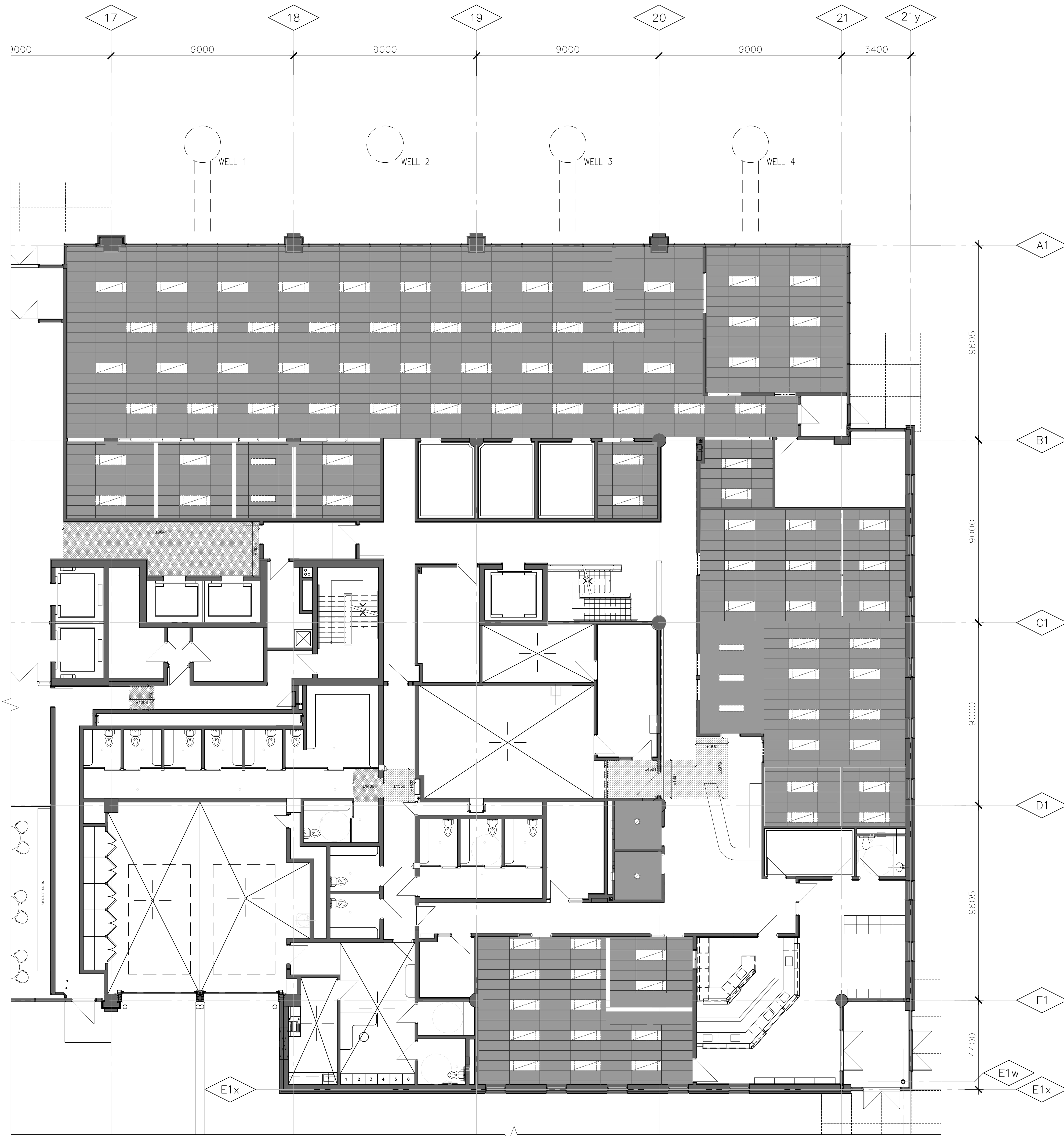
1 REFLECTED CEILING PLAN DEMOLITION- GROUND FLOOR SCALE: 1:100
