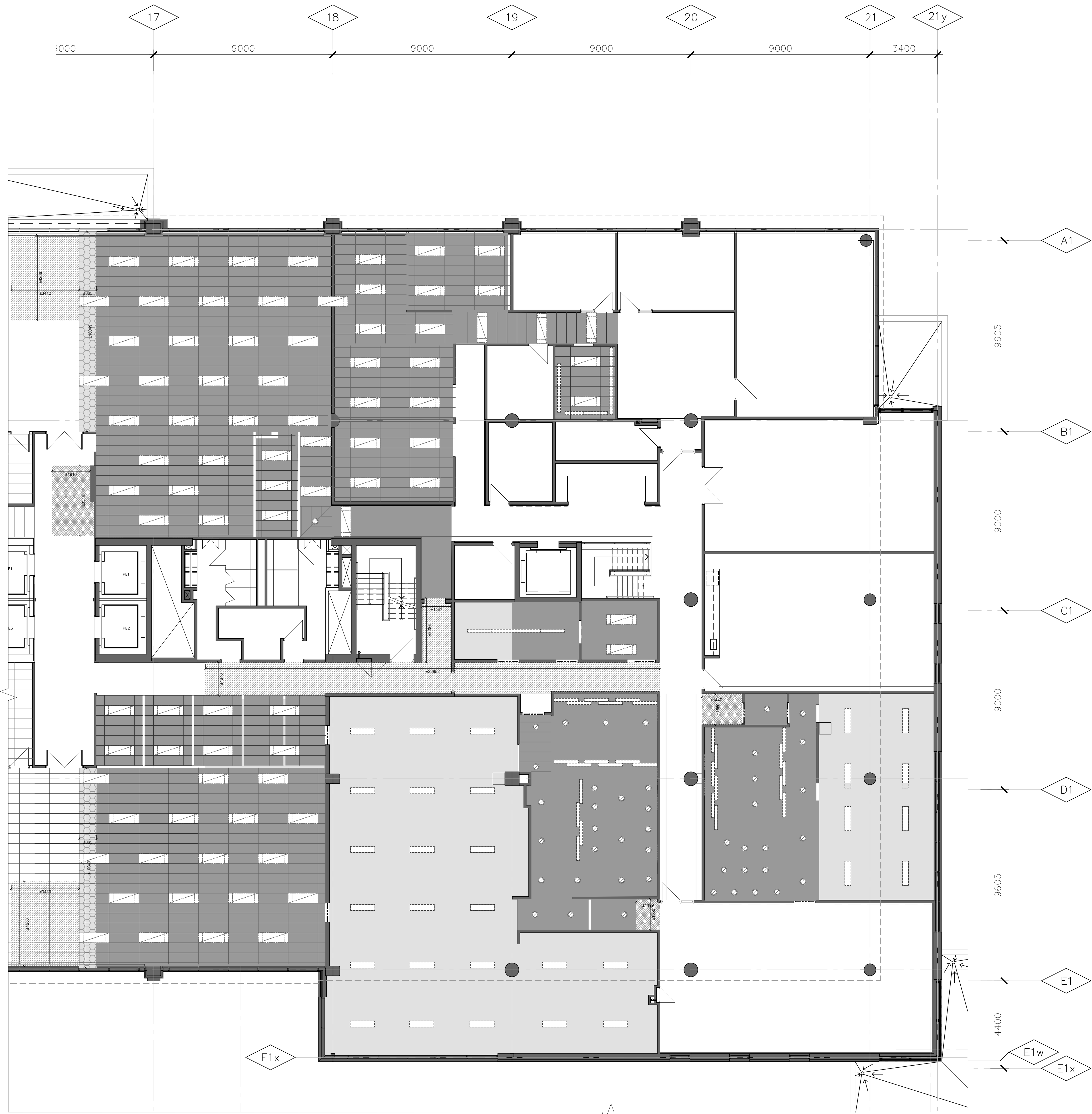
2 REFLECTED CEILING PLAN DEMOLITION- SECOND FLOOR SCALE: 1:100
